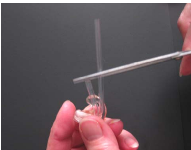
10. Cut the new tube to the same length as the old tube
