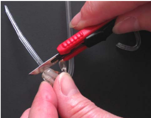
8. Cut off the tapered end of the tube with a sharp blade. Make sure there are no rough edges left.
