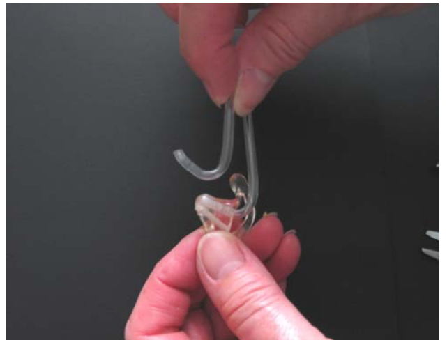
9. Use the old piece of tube as a guide as to the length that the new tube needs to be cut
