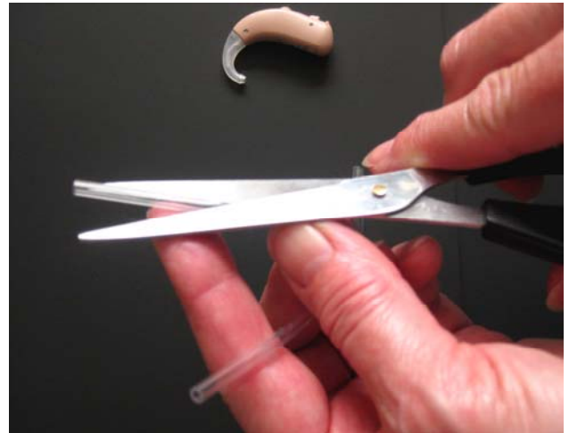
4. Taper the end of the new piece of tubing
